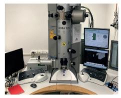
ultramicrotome for ultrathin sectioning of biological samples and with a Leica EMPG cryoplunging system for cryo-sample preparation.
